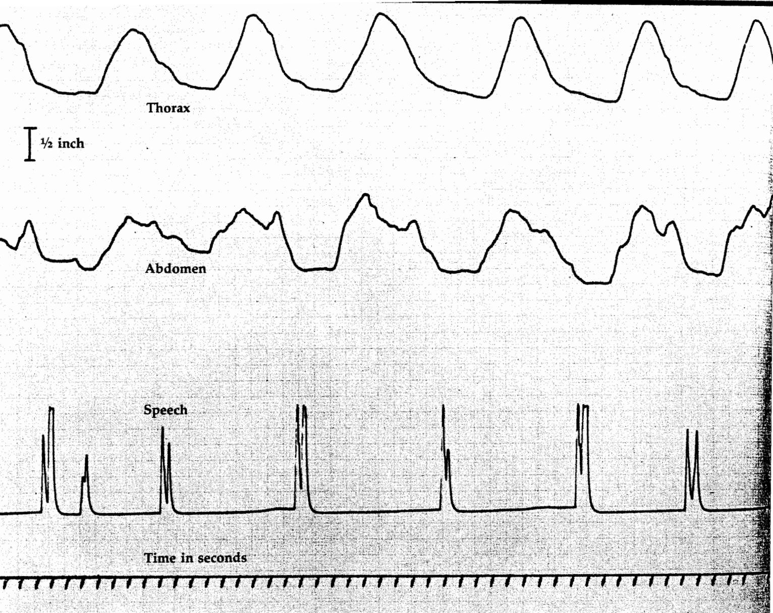
**Figure F.** *Pneumogram obtained with the portable impedance pneumograph. The top line represents the thorax; the second line, the abdomen. Calibration mark indicates one half inch circumference change; expansion is indicated by upward pen deflection. Third line shows speech (SPL), and the bottom line shows time, in one second intervals.*
