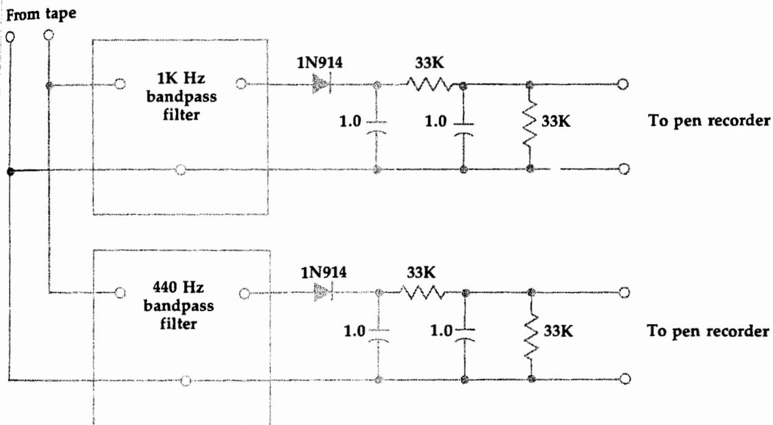
**Figure D.** Separator-demodulator circuit.  $C$  in  $\mu f$ ,  $R$  in ohms  $\pm 10$  per cent.
