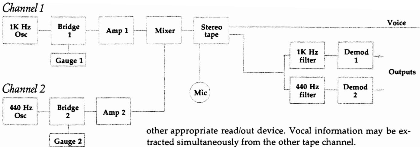
**Figure A.** Functional block diagram of a two-channel portable impedance pneumograph.
